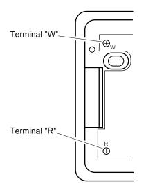
Figure 33 - Thermostat Base Terminals "W" and "R"
